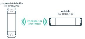
**104 + 101** Bridge mode is enabled after the device has been added to a 104 controller and a 101 power supply has been connected to the DALI terminals.
